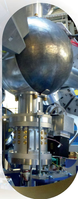
An early experiment using the AGATA detector at LNL showed that the calcium-42 nucleus, when set spinning, elongates into a triaxial 'super-deformed' state
