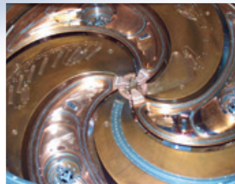
Proton therapy is carried out at the INFN Laboratory in Catania, Italy using a superconducting cyclotron to deliver the particle beam
