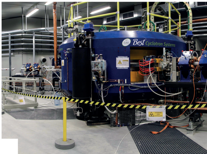
The newly built ISOLPharm radioactive ion beam facility in Legnaro, Italy specialises in making specialised medical radioisotopes. It employs a compact cyclotron. [Credit INFN LNL].
