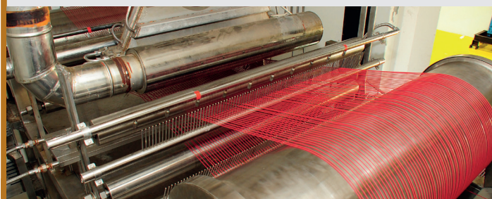
Cables being irradiated in Malaysia to improve their resistance and longevity. [Credit IAEA].
