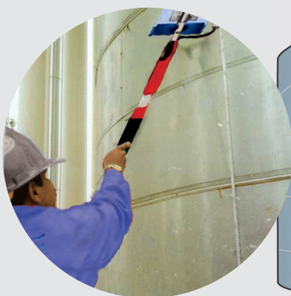
Levels and interfaces in feedstocks in storage tanks can be evaluated using a neutron gauge. [Credit Scantech Nuscan].
