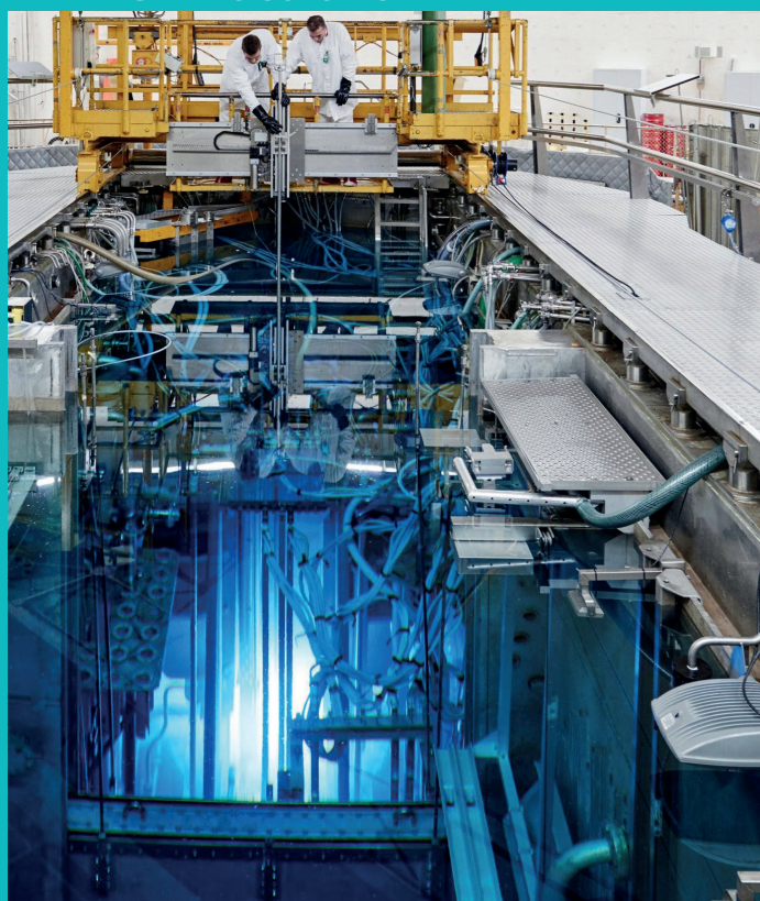
■ The High Flux Reactor at Patten in the Netherlands, which produces a range of medical isotopes such as molybdenum-99. [Credit NRG].
