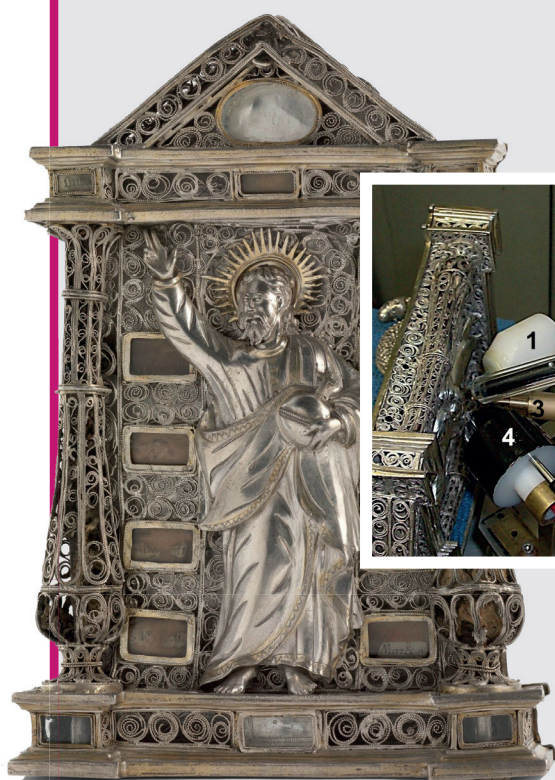
■ Left: The pax of the Vidigueira treasure; right: The pax being analysed with a proton beam. 1: X-ray detector; 2: camera; 3: beam exit nozzle; 4: particle detector; 5: lasers [Credit The Centre for Nuclear Sciences and Technologies, Instituto Superior Técnico, Portugal].
