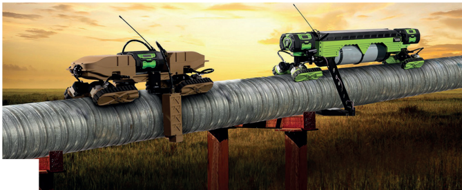
Radiographic-testing crawlers to detect corrosion and oil flow in pipelines. [Credit Mistras].
