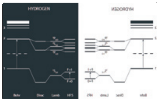
Precision experiments at CERN aim to search for minute differences in the quantum energy levels of hydrogen (proton, electron), antihydrogen (antiproton and positron) that might indicate CPT symmetry-breaking
